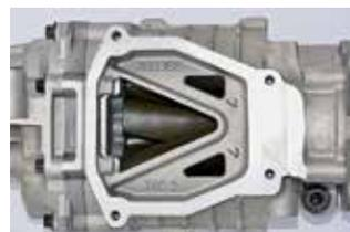
The M45's restricted inlet. Porting has no noticeable power!
