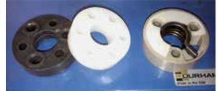
On the subject of DIY kits, it's obvious that this is a mechanical rebuild requiring bearings that are pressed out of the main casing. The seals too have to be installed so they sit correctly. "The M45 uses captive seals and bearings in the PTO gearbox that must be machined out to replace—a machine shop-only job," says Dustin.
