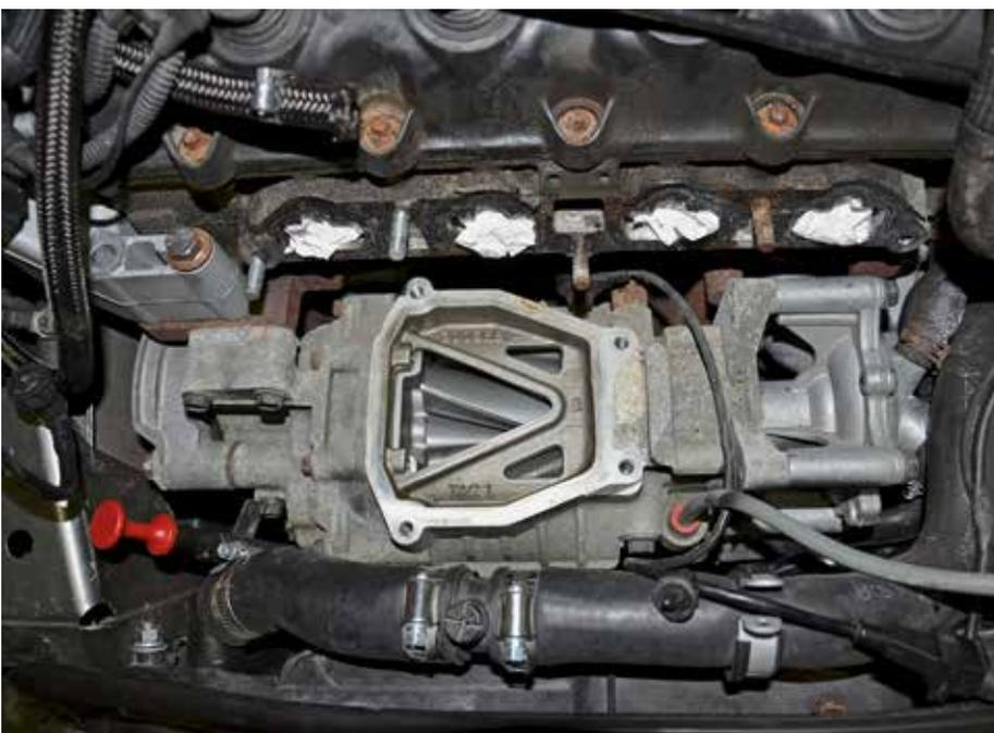
In position, the PTO drives the water pump to the right.
